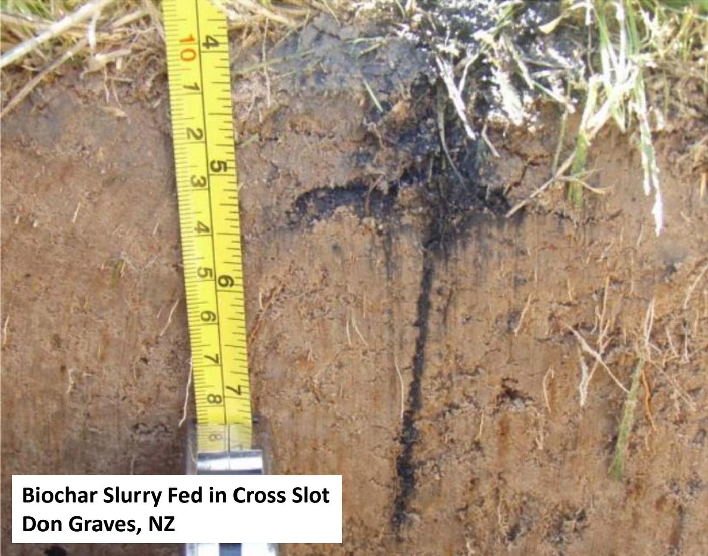
**Biochar Slurry Fed in Cross Slot
