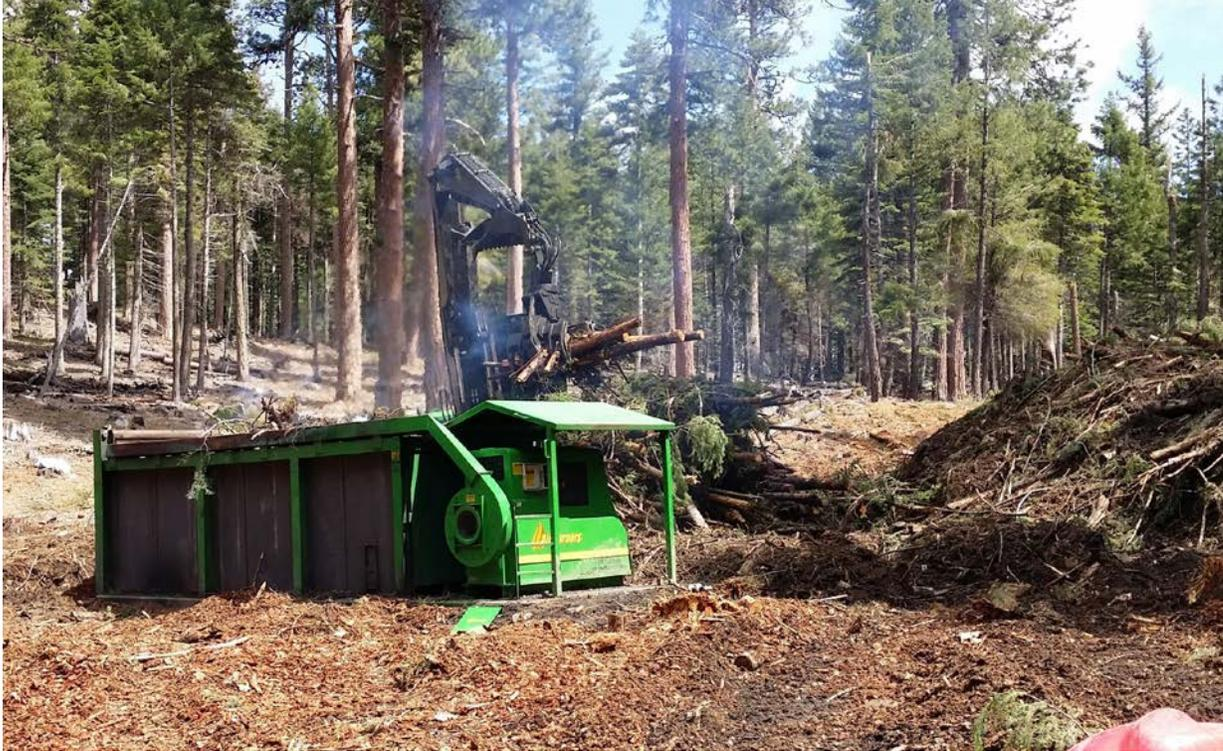
**Roll off refractory lined “Air Curtain Burner” making biochar from forest residues, Oregon**
